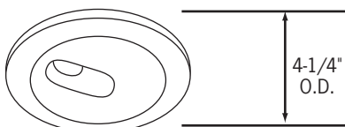
CTR303NMH-P Slotted Wall Wash 1-3/8" x 2-1/2" Oblong Slot 50° Swing adjustment, external 358° rotation. Slot aperture permits maximum beam area adjustment for either wall wash or concealed accent lighting effects. Black interior surface, (1) 45mm lens option.
